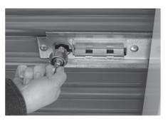
**STEP 5:** To lock the door, reinsert the cylinder with the key in a vertical position and the flat side of the cylinder facing towards the ground.
