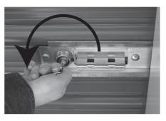
**STEP 6:** Turn the key counterclockwise 90 degrees so the key is once again horizontal in your hand and pull the key from the lock.
